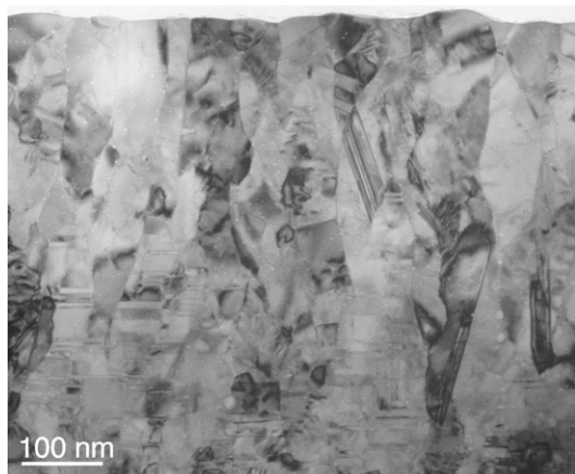
Fig. 5. TEM cross-section of the same film as in Fig. 3. Although the point defects and many of the twin boundaries are annealed out, the lateral grain size remains around 50 nm.
